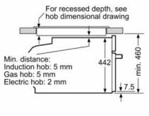
measurements in mm
