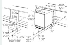
\* variable base/substructure height
