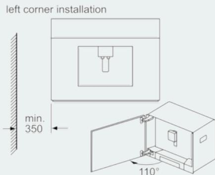
If using the 92° hinge limiter (spare part no. 00636455), the minimum distance to the wall is only 100 mm.
