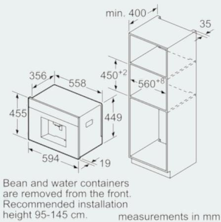
Bean and water containers are removed from the front. Recommended installation height 95-145 cm.
